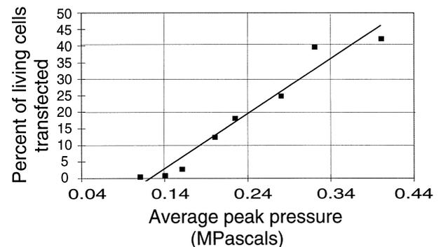
Fig. 5. Transfection rate of living cells after ultrasound exposure as a function of average peak pressure of the 20-s burst of 1.0-MHz ultrasound. The DNA concentration was 40  $\mu\text{g/mL}$  and the AlbuNex<sup>®</sup> concentration was  $50 \times 10^6$  bubbles/mL prior to exposure. Continuous line is best linear fit.
