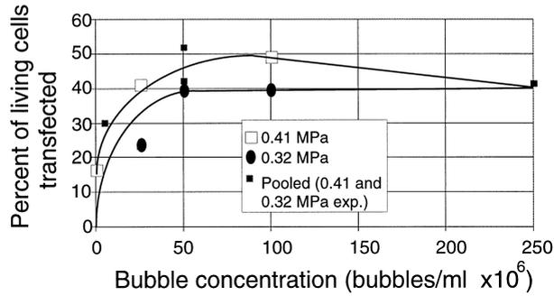
Fig. 3. Transfection rate of living cells after exposure plotted against AlbuNex<sup>®</sup> concentration at the time of exposure. Exposure time is 20 s at the indicated average peak pressure. Pooled data were from a separate experiment. Continuous lines are hand drawn.
