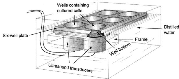
Fig. 1. Apparatus used to expose cells. A 35-mm-diameter 1.0-MHz transducer was placed 2 mm below each of two wells of a six-well culture plate. The experiment was conducted within a water bath maintained at 37°C. Water completed the acoustic coupling with the bottom of the culture plate. [Reproduced with permission from Kim et al. (1996)].
